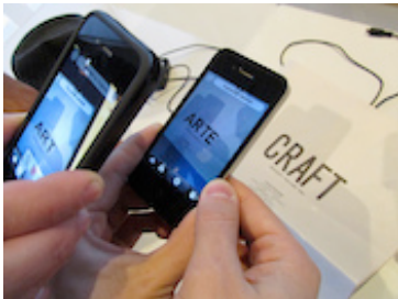
Figure 1: An example of AR functionality within a single application on a traditional platform, WordLens does real-time in-image translation. (Image copyright: Neven Mrgan. Image source: http://www.flickr.com/photos/neven/5269418871/ )
